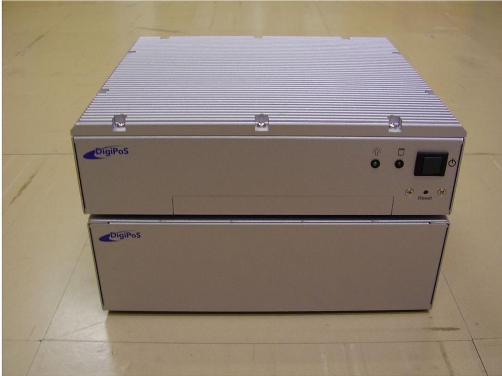
**Figure 15** Front view of PH6000T System Unit showing Main system unit (top) and IO Expansion Hub (bottom)
