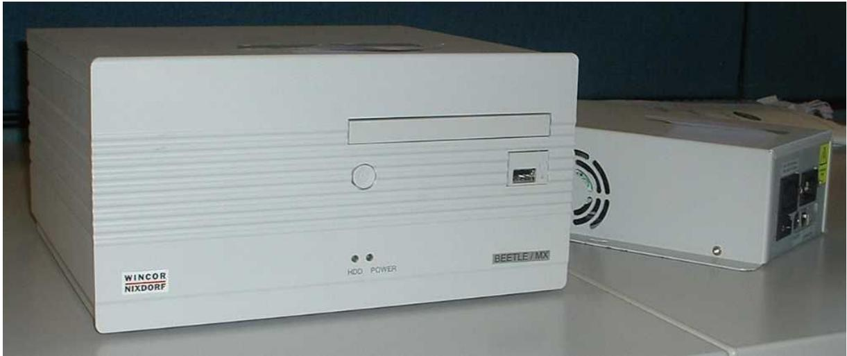
**Figure 11 BEETLE-X POS terminal with external power supply unit**
