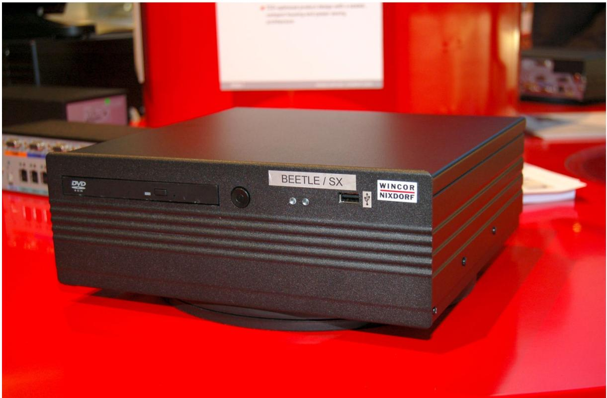
**Figure 12 BEETLE-SX POS terminal**
