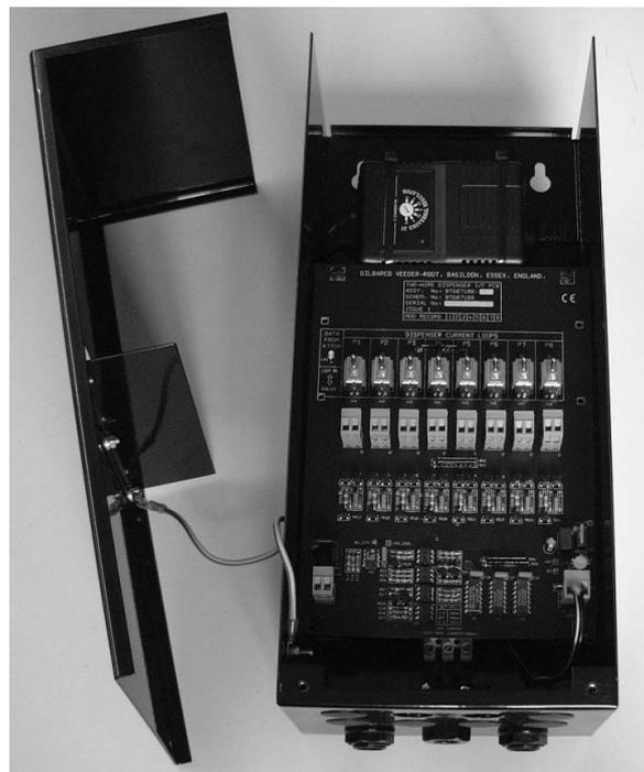
**Figure 16** Top view of BW703635-103 DDM with generic 2-Wire Dispenser Interface PCB
