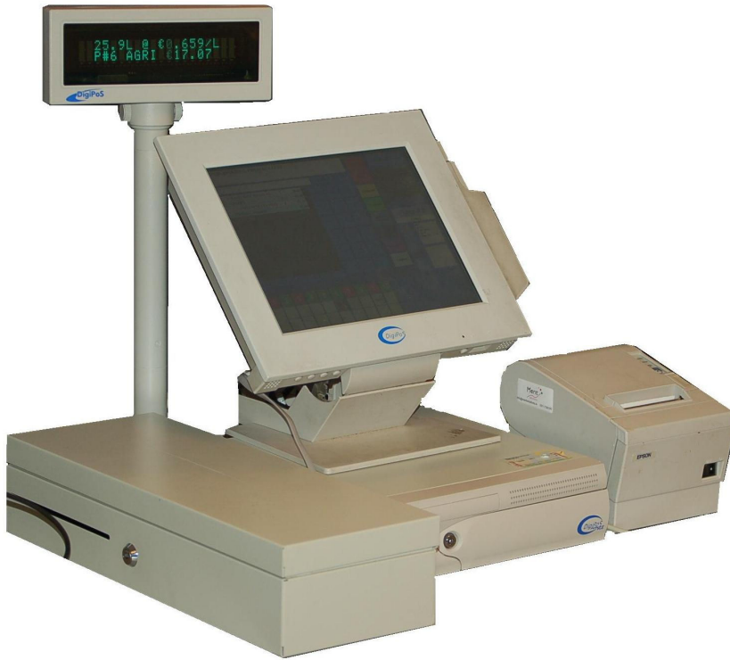
Figure 11 DigiPos PowerPos machine with line display, cash drawer and printer
