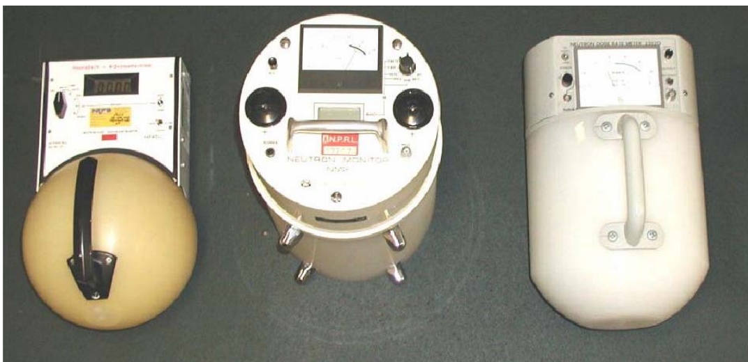
FIGURE 1 The three designs of instrument modelled in the earlier work and in this project: the Leake (0949) on the left, the NM2 in the centre and the Studsvik 2202D on the right
