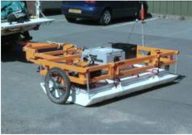
Figure 2 - Ground-penetrating radar being towed behind a vehicle
