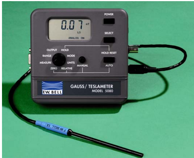
FIGURE 2.7 Commercially available Hall effect probe and read-out
