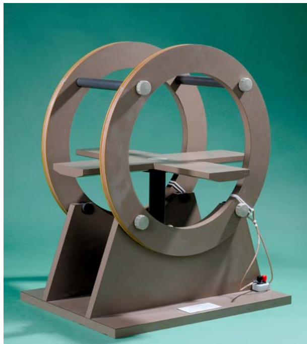
FIGURE 2.8 Helmholtz coils used for calibration of magnetic field sensors
