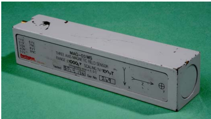
FIGURE 2.6 Commercially available fluxgate magnetometer (of dimensions 15 \times 3 \times 3 \text{ cm}^3 )
