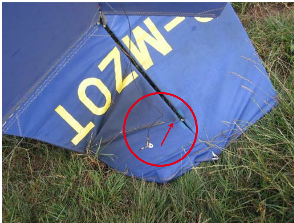
As-found tailplane bracing wires: arrow indicates attachment point on fin
