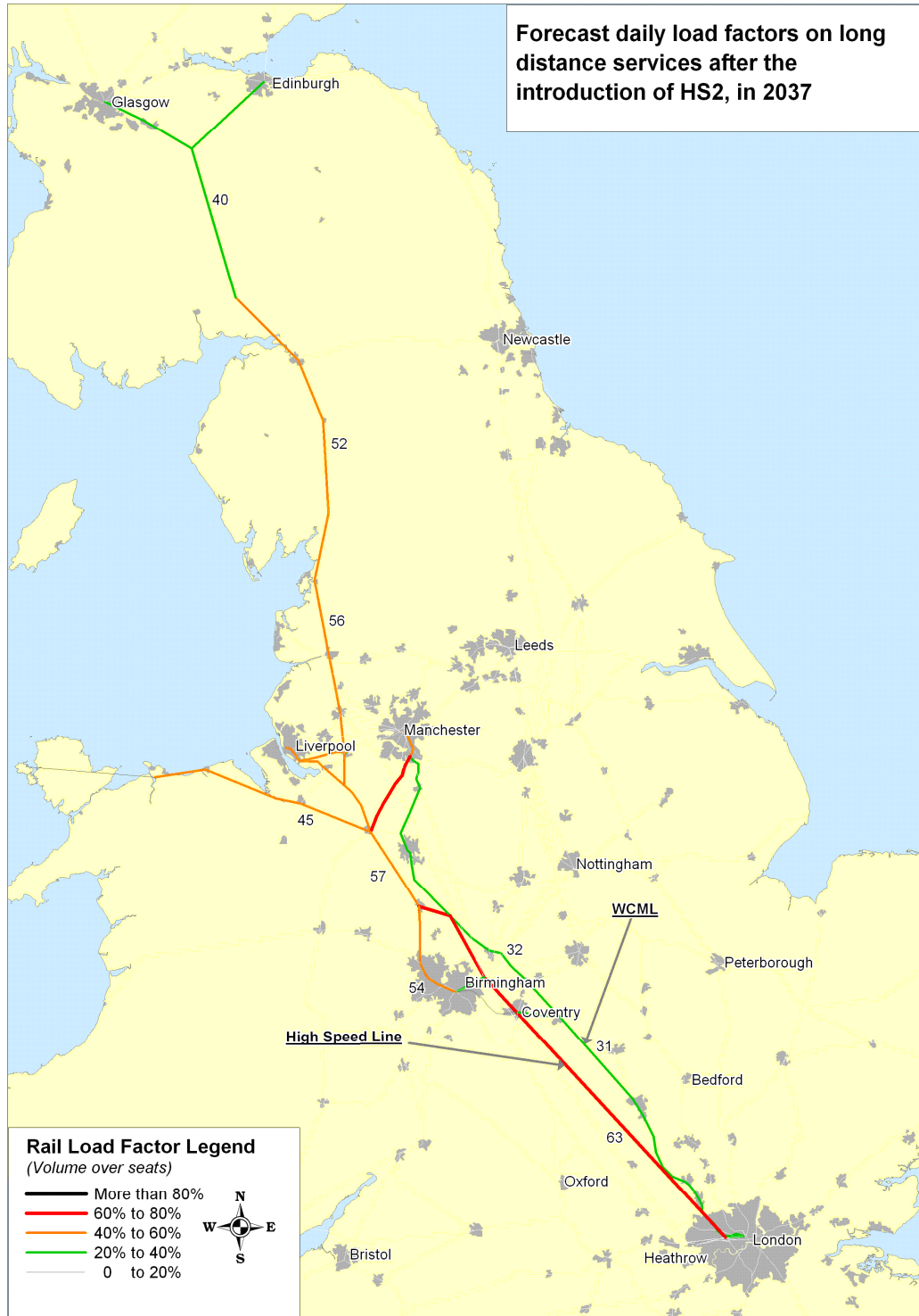
Figure 5.2 Long Distance Weekday Load Factors in 2037 – with HS2 London to Birmingham (Phase 1), % of seats occupied
