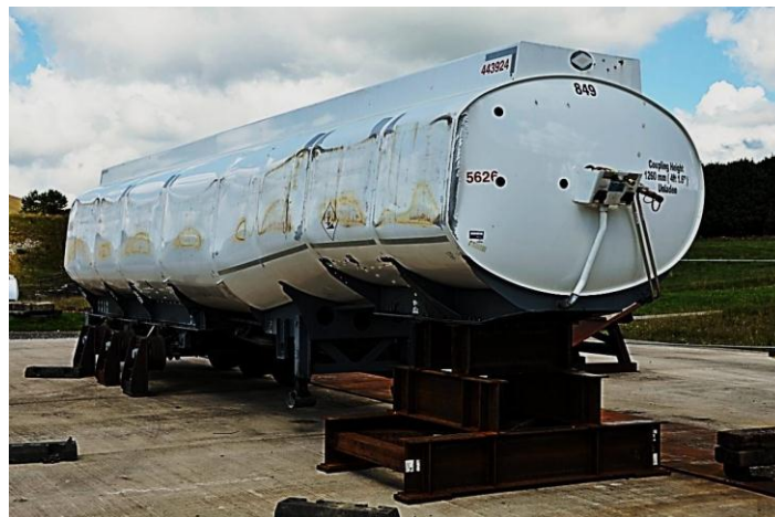
Figure 11. Impact damage to a non-compliant tanker, viewed from front
