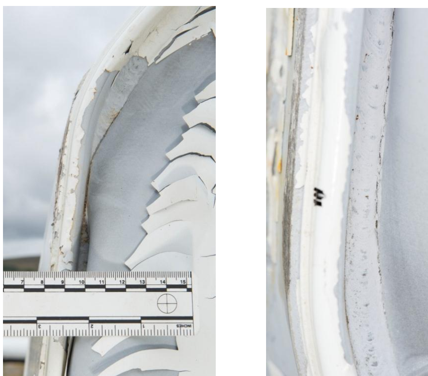
Figure 14. The 2011 tanker – rupture at toe of weld at top of impact zone (left) and crack at toe of weld at bottom of impact zone (right).
