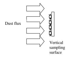
If the flux gauge is located on the site perimeter, then the flux that is measured is the fugitive dust release rate across the site boundary.
