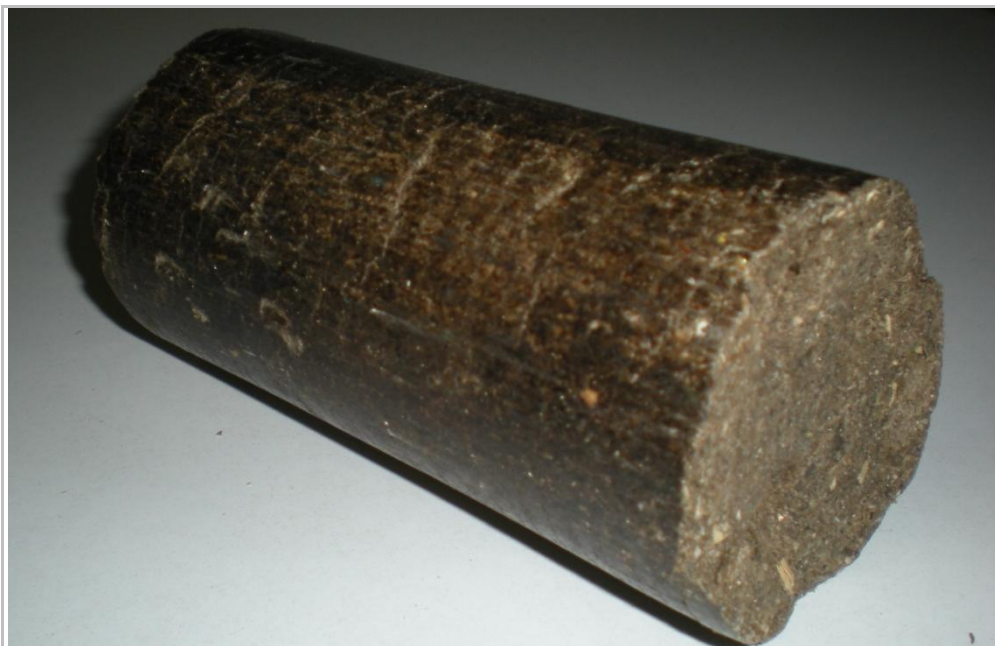
Figure 3: A compacted BioFibe 'log' prior to pyrolysis (note that this material has been subject to significant testing and proven to contain very low levels of inorganic material or contaminants.)
