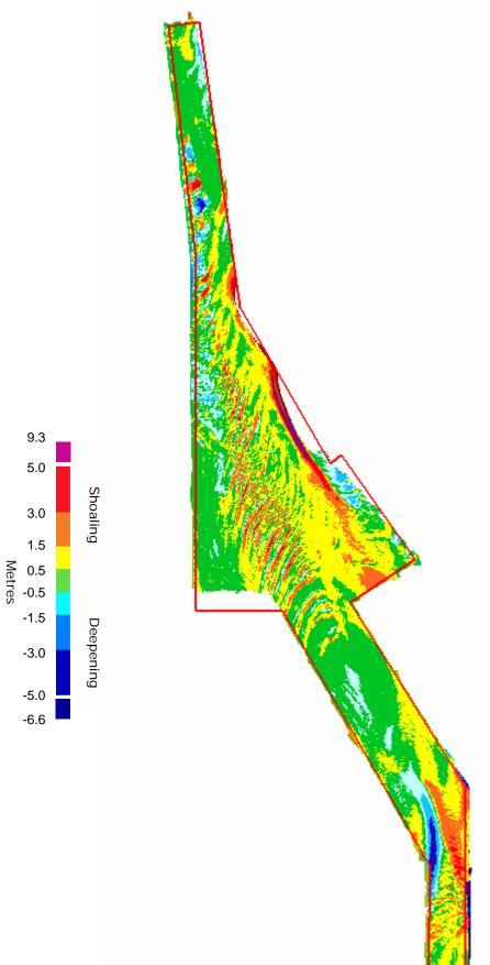
SURFACE FROM THE 2013 SURVEY AND CROSS-SECTIONS FROM THE 2012 AND 2013 SURVEYS
