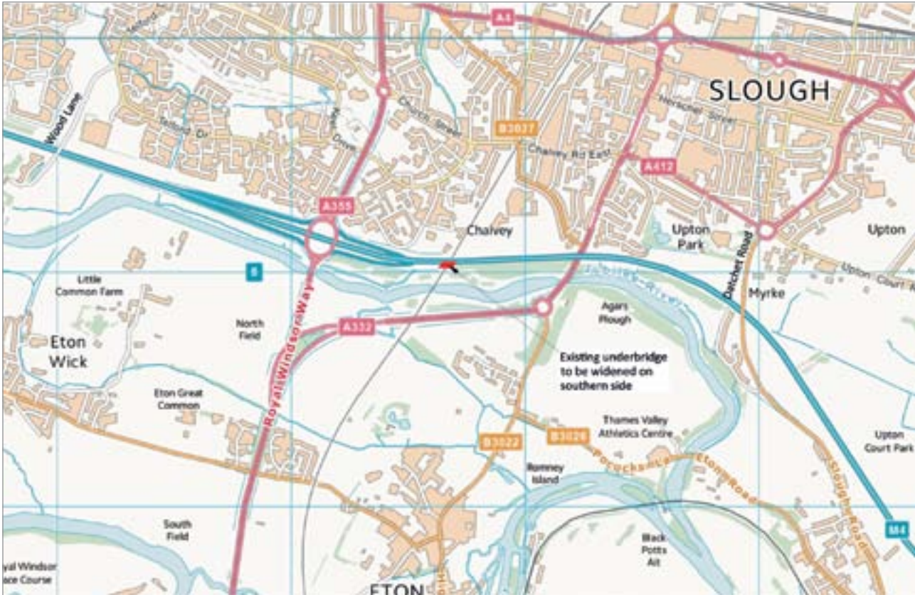
Figure 20: Windsor Rail underbridge
