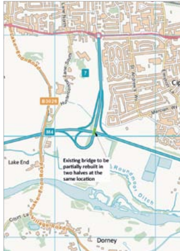
Figure 12: Junction 7 Huntercombe Spur overbridgebridges
