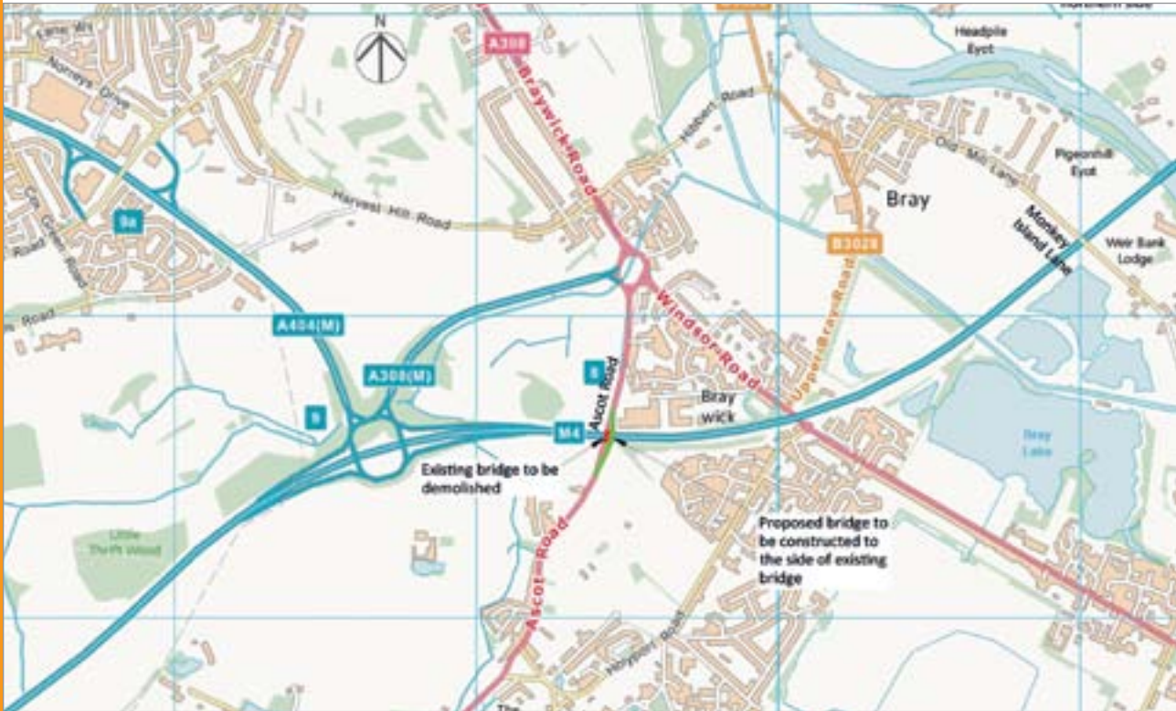
Figure 9: Ascot Road overbridge
