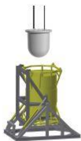
The Container lid is removed and RPV is loaded into container
