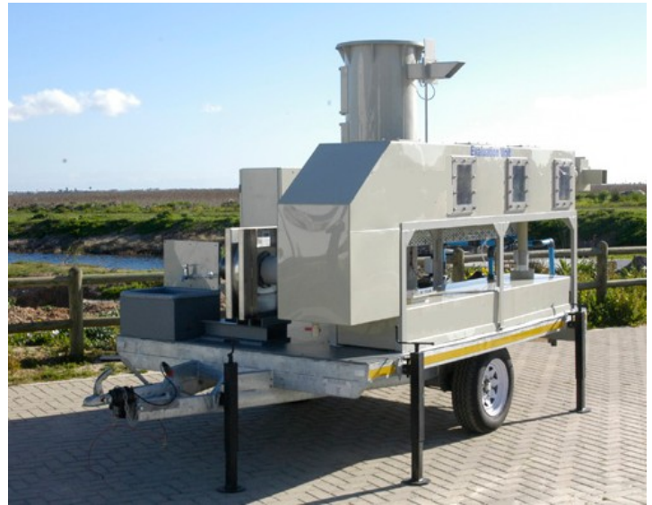
Our 700m 3 /hr Evaluation Unit is available for trial installations. This is a fully functional 2 phase unit.
