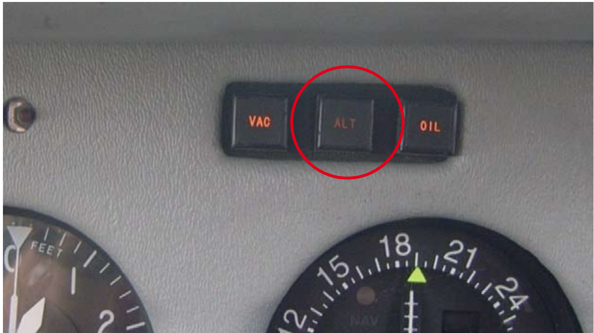
Figure 1 Alternator fail warning light
