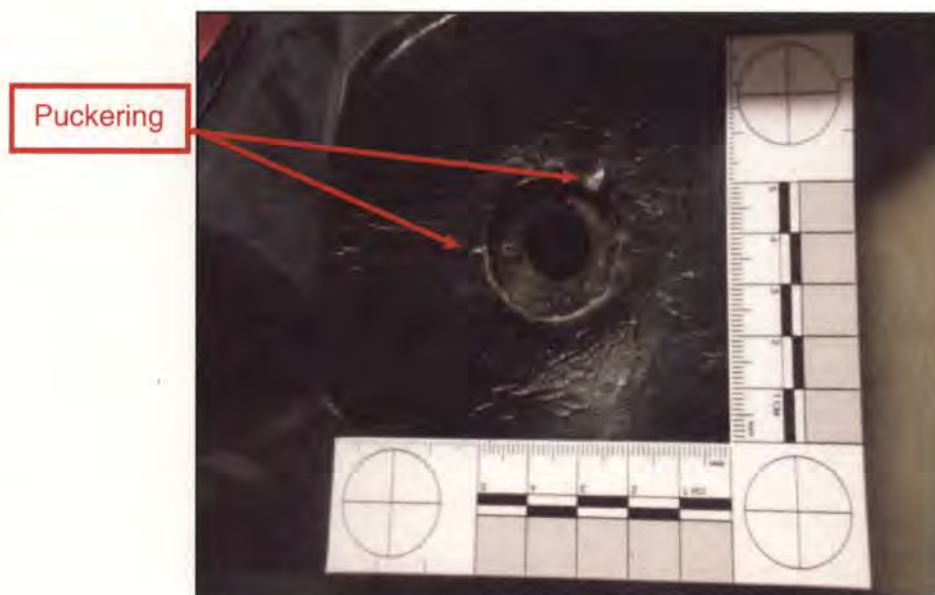
Figure 59. Rubber Section of Valve Assembly retained in Liferaft.
