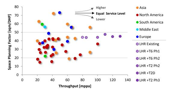
Figure 8-1 Space Planning Factor for Airports with more than 20 mppa, Showing All Phases of the Proposed Scheme
