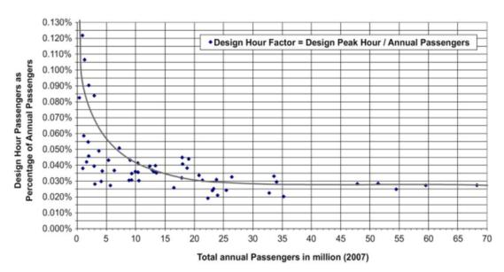
Figure 2-1 Relationship Between Annual Capacity and Design Hour (Source: Airport Evolution and Capacity Forecasting, Bubalo, 2011)
