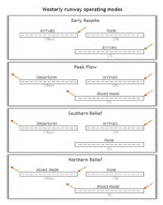
Figure 3-2 Heathrow Airport Extended Northern Runway Concept of Operating Modes (Source: Heathrow Hub Ltd submission to the Airports Commission)
