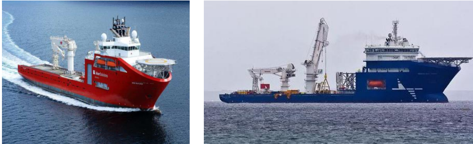
Figure 34: Dynamic Positioning (DP) vessels deployed at EMEC’s tidal test site to install tidal turbines and support structures
