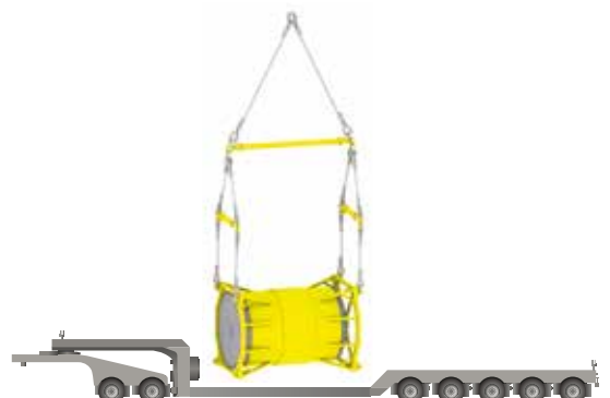
The Container is lifted onto transport trailer
