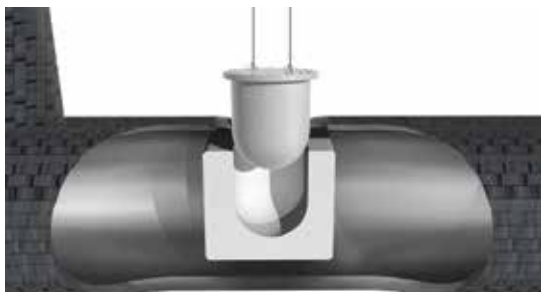
RPV is lifted out of submarine
