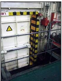
While the passenger ferry *Eurovoyager* was en-route to Ramsgate, UK, from Ostend, Belgium, an engine fitter was trapped for almost 4 minutes in a hydraulically operated steel watertight door in the engine room. He sustained major crush injuries and was airlifted to a London hospital shortly after the ferry arrived in Ramsgate.
