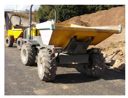
When being loaded dumpers should be switched off, the keys removed and the driver on the ground in a safe position.
