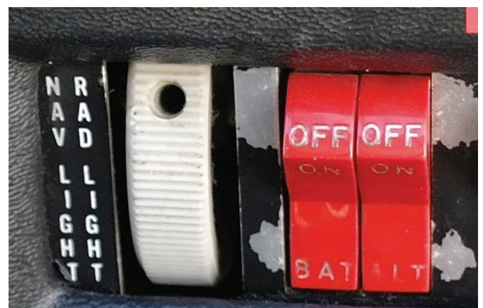
Figure 5 Battery master and alternator switches (red)
