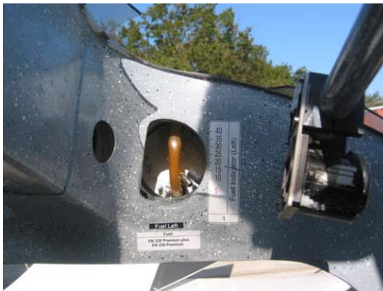
View of left tank fuel contents sight tube and gauge
