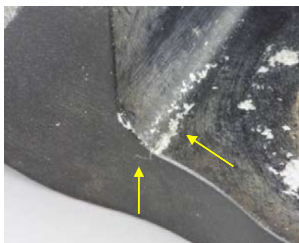
Figure 4 Cracking at base of lugs
