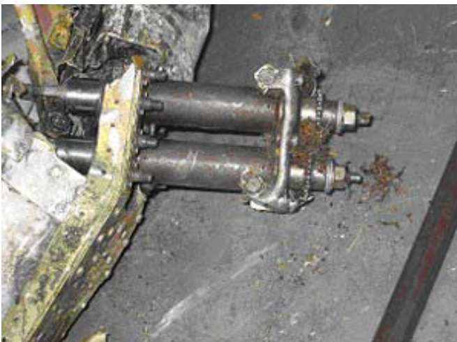
Right elevator trim jack
