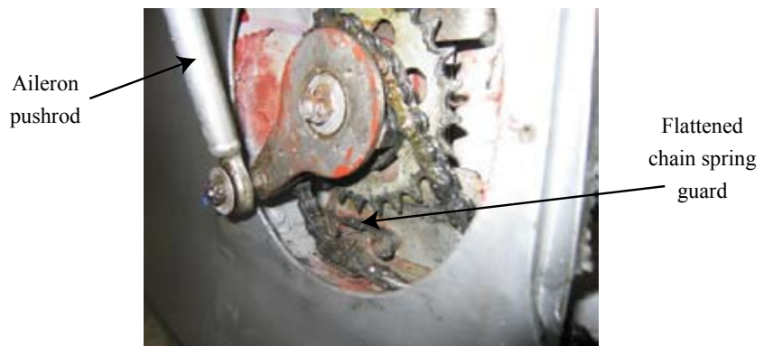
Figure 2 Photograph showing derailed aileron chain in lower left mainplane
