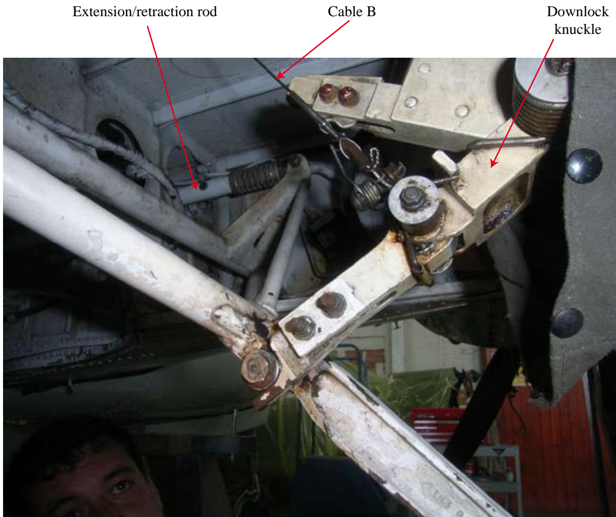
Figure 1 Gear down and locked
