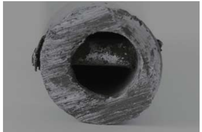
Figure 6 Detail of failed scroll pin in pivot shaft
