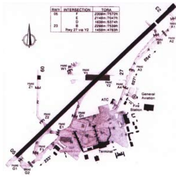
Figure 4 Cross Runway operations
