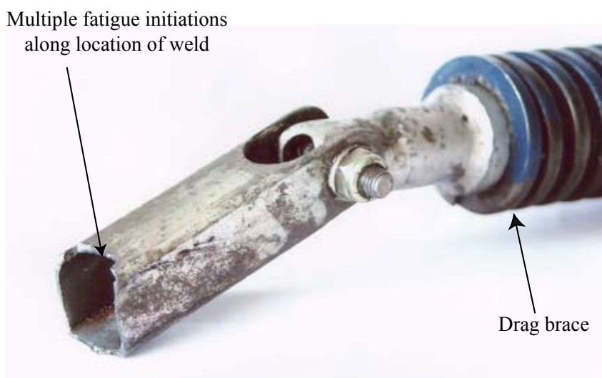
Figure 2 Failed engine mount tubing for G-BUDI
