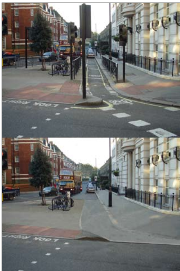
Fig. 3.24 Visualisation (lower image) showing an alternative approach to providing for cyclists alongside a signalised junction.
