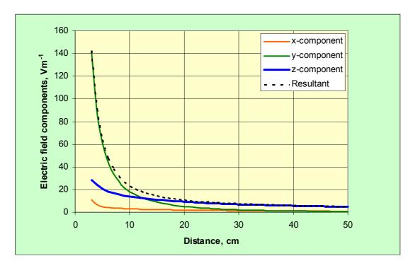
Figure A1 The components of electric field strength and the resultant as a function of distance along the negative y-direction at x = 3 cm- and z = 9 cm
