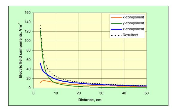
Figure A21 The components of electric field strength and the resultant as a function of distance along the negative *y*-direction at x = 3 cm and z = 9 cm
