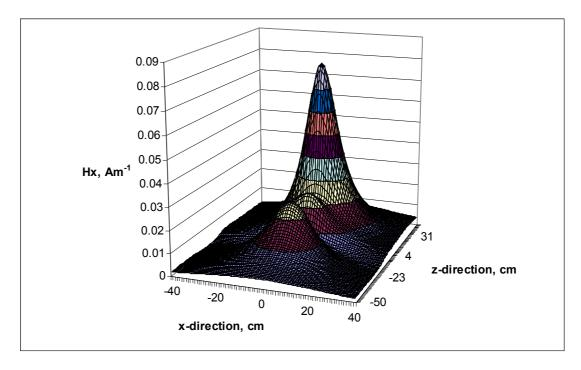
Figure A17 The x-component of magnetic field as a function of x and z at a displacement of 7 cm from the transponder along the negative y-direction
