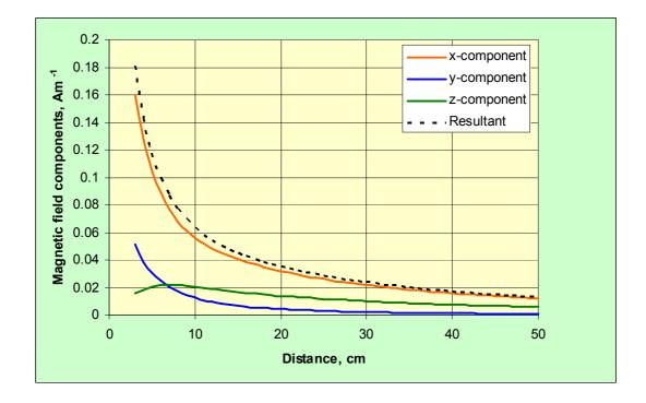
Figure A22 The components of magnetic field strength and the resultant as a function of distance along the negative y-direction at x = 3 cm and z = 9 cm
