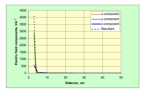
Figure A4 The components of electric field strength and the resultant as a function of distance along the positive x-direction at y = 0 cm and z = 5 cm
