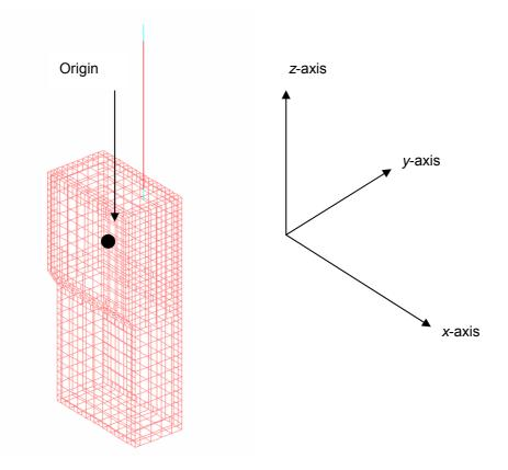
Figure 5 NEC model of the Mode S transponder with a monopole antenna
