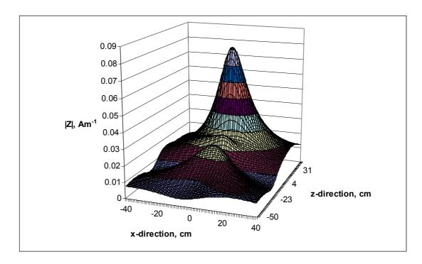
Figure A20 The resultant magnetic field as a function of x and z at a displacement of 7 cm from the transponder along the negative *y*-direction
