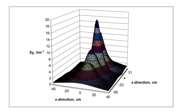
Figure A8 The y-component of electric field as a function of x and z at a displacement of 7 cm from the transponder along the negative y-direction
