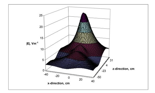
Figure A10 The resultant electric field strength as a function of x and z at a displacement of 7 cm from the transponder along the negative *y*-direction
