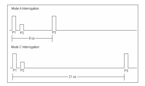
Figure 1 Mode A/C Interrogation pulses transmitted from an SSR ground station
