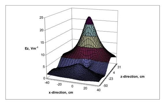
Figure A9 The z-component of electric field as a function of x and z at a displacement of 7 cm from the transponder along the negative y-direction
