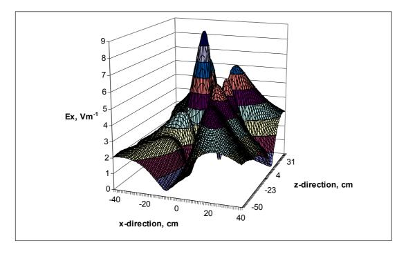
Figure A7 The x-component of electric field as a function of x and z at a displacement of 7 cm from the transponder along the negative y-direction
