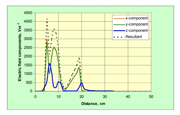
Figure A5 The components of electric field strength and the resultant as a function of distance along the positive z-direction at x = 3 cm and y = 0 cm
