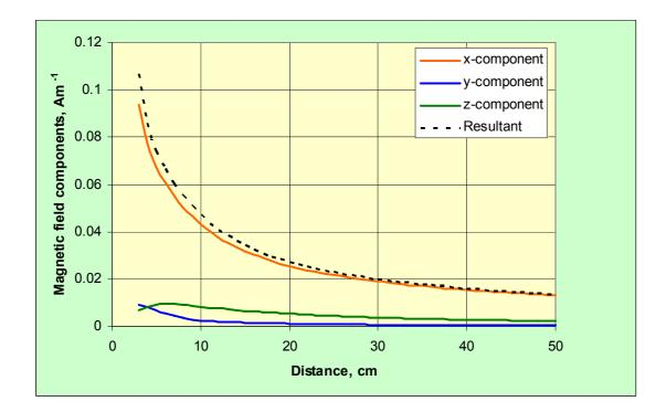
Figure A12 The components of magnetic field strength and the resultant as a function of distance along the positive *y*-direction at x = 3 cm and z = 9 cm
