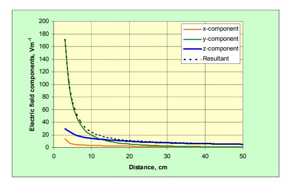
Figure A2 The components of electric field strength and the resultant as a function of distance along the positive y-direction at x = 3 cm- and z = 9cm
