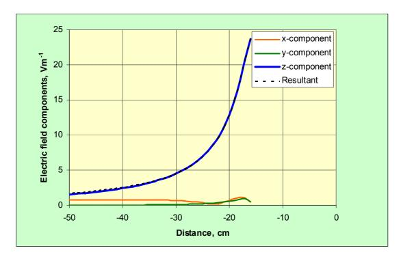
Figure A6 The components of electric field strength and the resultant as a function of distance along the negative z-direction at x = -2 cm and y = 0 cm
