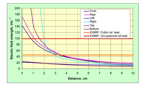
Figure 6 Electric field strength as a function of distance from various sides of the transponder in relation to the ICNIRP reference levels
