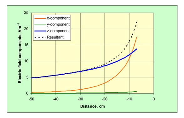
Figure A3 The components of electric field strength and the resultant as a function of distance along the negative x-direction at y = 0 cm and z = 5 cm
