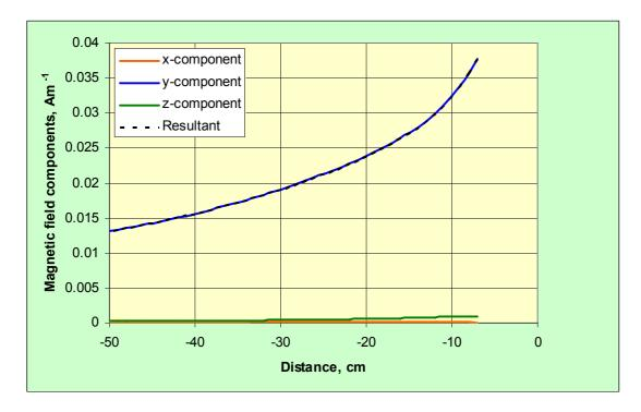
Figure A13 The components of magnetic field strength and the resultant as a function of distance along the negative x-direction at y = 0 cm and z = 5 cm
