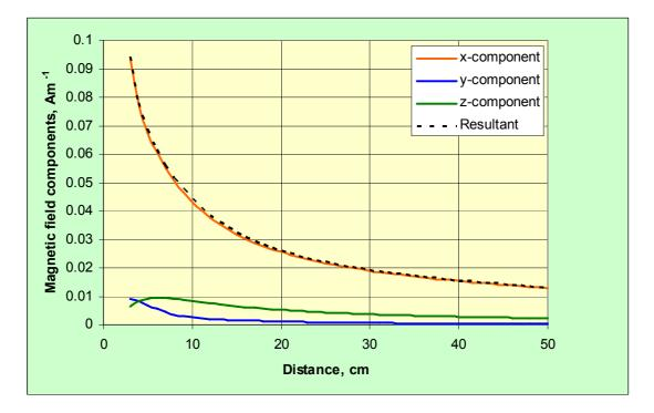
Figure A11 The components of magnetic field strength and the resultant as a function of distance along the negative *y*-direction at x = 3 cm and z = 9cm
