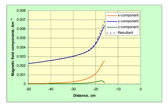
Figure A16 The components of magnetic field strength and the resultant as a function of distance along the negative z-direction at x = -2 cm and y = 0 cm
