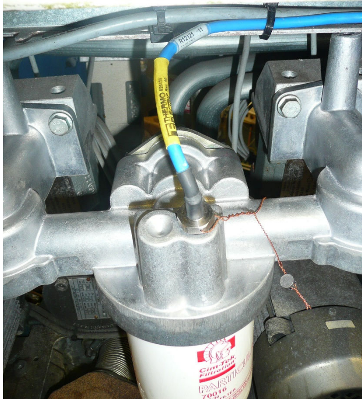
Figure 7 Example Mounting of Temperature Probe
