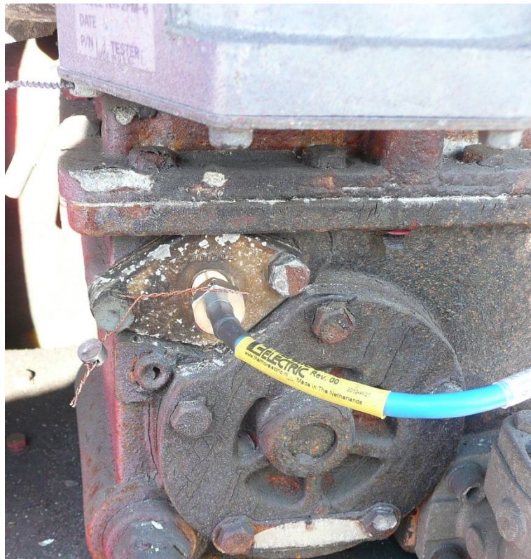
Figure 10 Example Mounting of Temperature Probe
