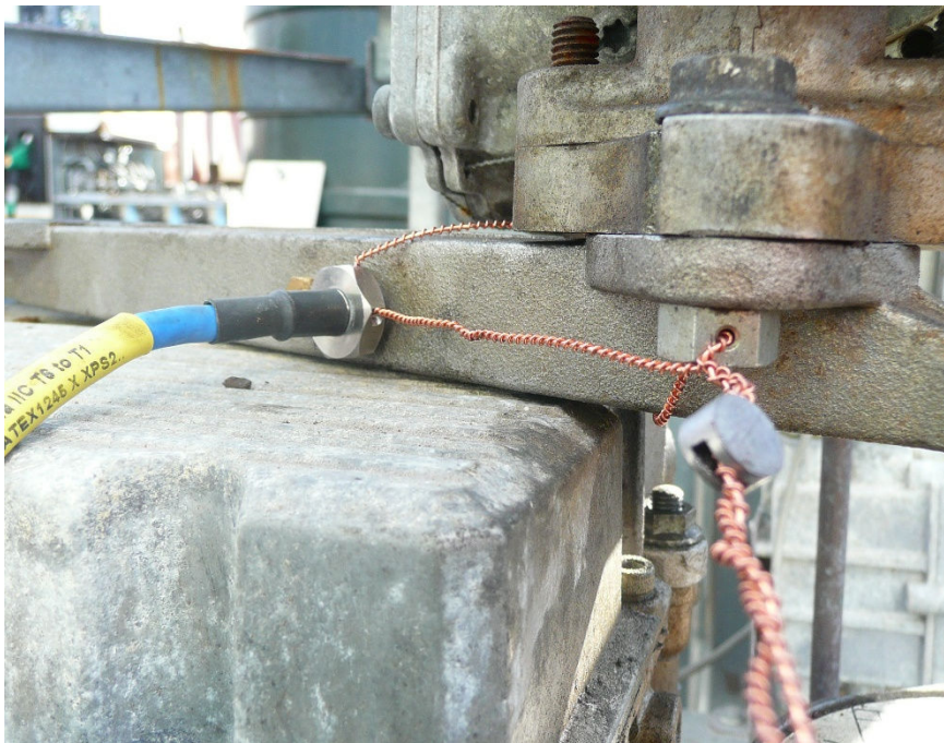
Figure 8 Example Mounting of Temperature Probe
