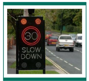
Figure 3 Vehicle activated VMS with flashing amber lamps
