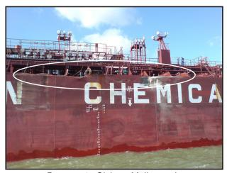
Damage to Sichem Melbourne's sheer strake and deck edge
