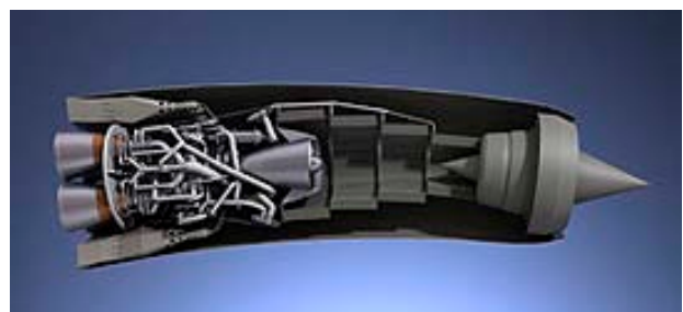
Synergetic Air-Breathing Rocket Engine. Credit: Reaction Engines Limited
