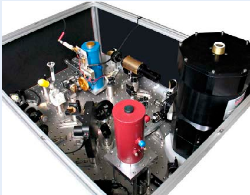
Breadboard of the first generation LHR. Credit: CEOI
