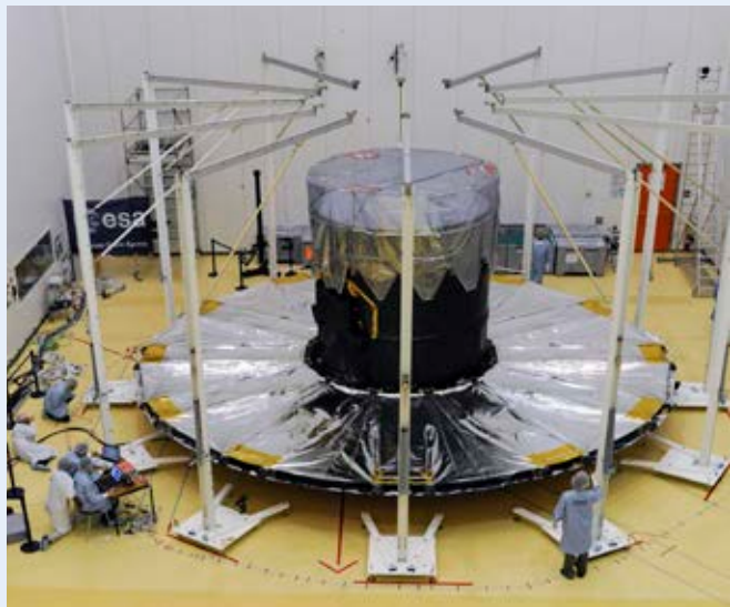
The Gaia spacecraft after the last deployment test of the sun shield. Credit: ESA
