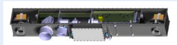
PanCam design (Credit: C.Theobald, MSSL)
