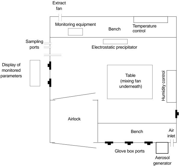
FIGURE 1 The Health Protection Agency radon chamber
