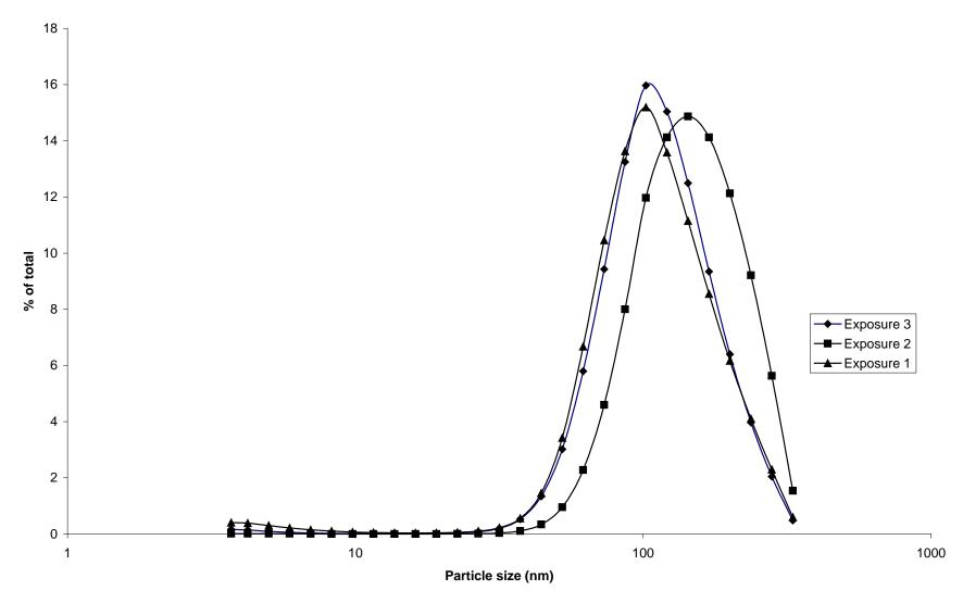
FIGURE 7 Ambient aerosol size distributions during exposures 1, 2 and 3
