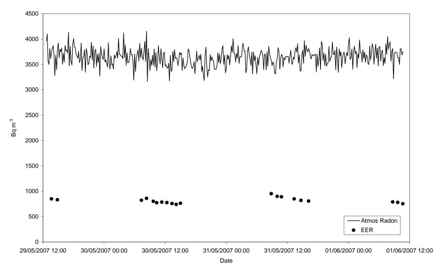
FIGURE 3 Radon and EER concentrations exposure 1
