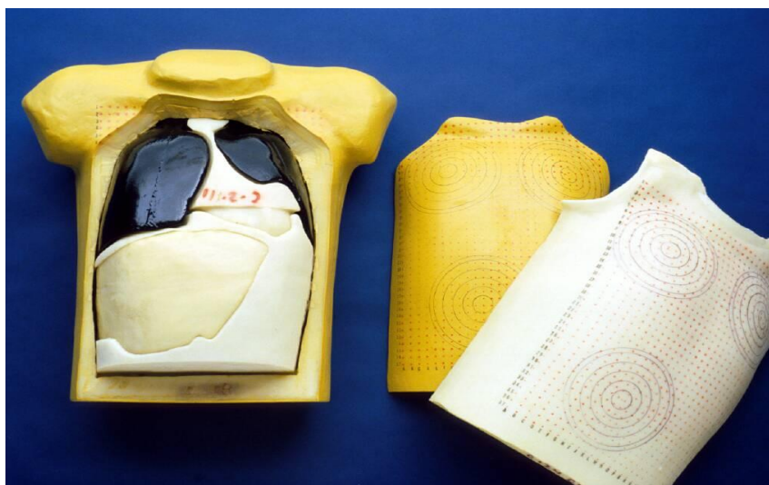
FIGURE 2 Lawrence Livermore realistic thoracic phantom showing internal organs (lungs in black, liver to lower left), standard chest wall and one overlay
