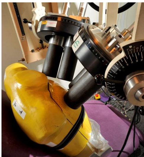
FIGURE 3 Phantoms arranged on chair for lung measurement showing position of GEM-FX detectors in relation to the Lawrence Livermore phantom with no overlay
