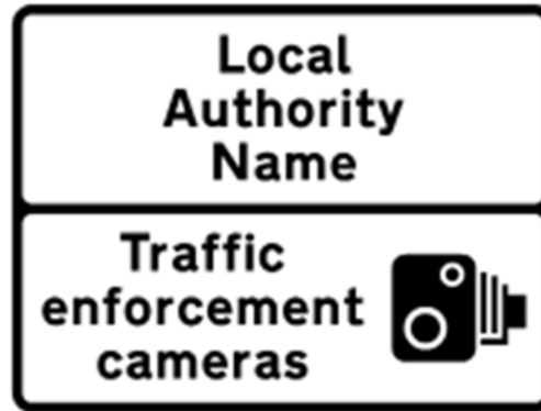
Figure 7.4 Example design of new sign including additional information on operators of enforcement cameras
