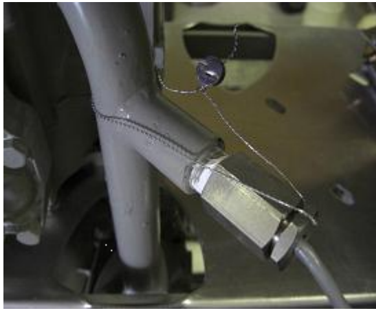
Figure 29 Typical installation of temperature sensor and sealing arrangement
