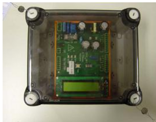
Figure 28 TVC unit sealing arrangement
