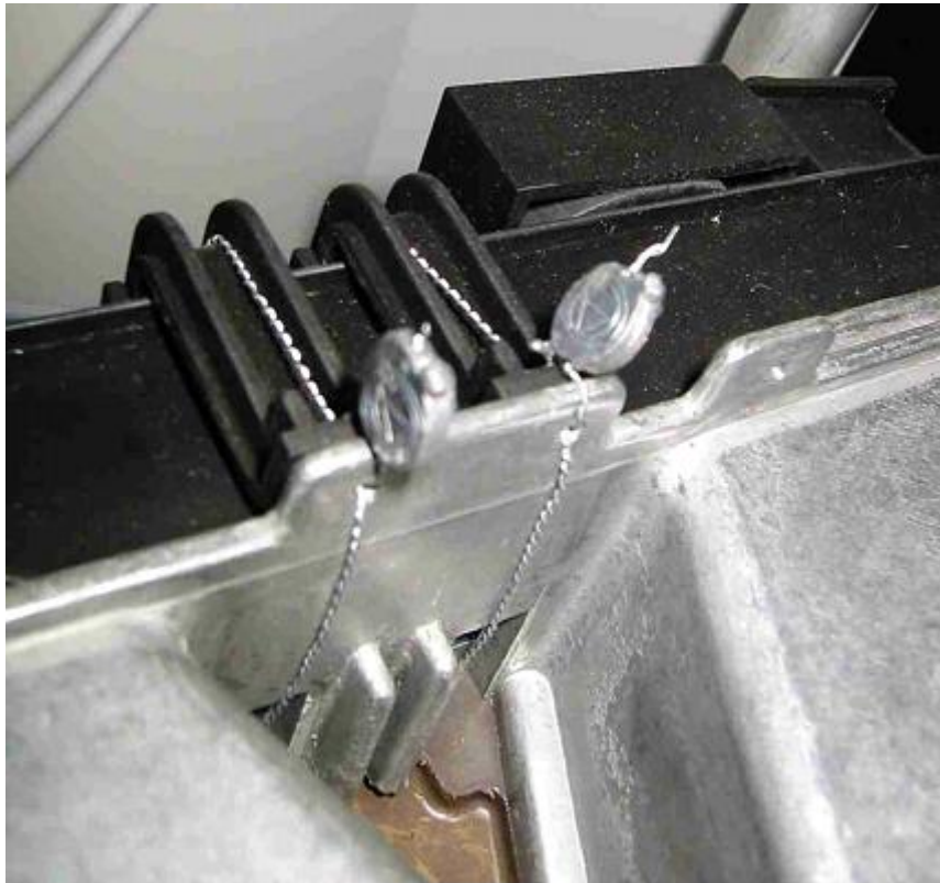
Figure 4 Sealing of Wayne Integrated Pulser (WIP)
