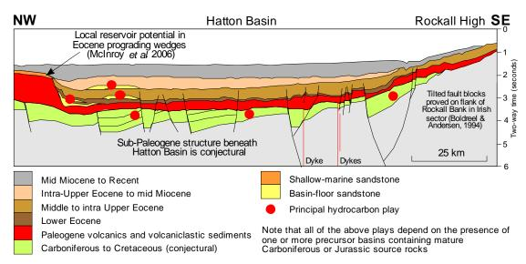
Fig. 25 Schematic play diagrm for the Hatton Basin. See Fig. 20 for location
