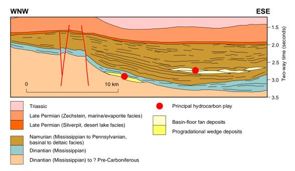
Fig 16 Geoseismic section illustrating undrilled Lower Carboniferous plays, North Sea Gas Province (adapted from Cameron and Ziegler 1997). See Fig. 14 for location
