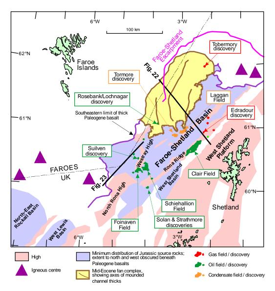
Fig. 21 Structural elements and location of mid Eocene fan complex, Faroe-Shetland Basin
