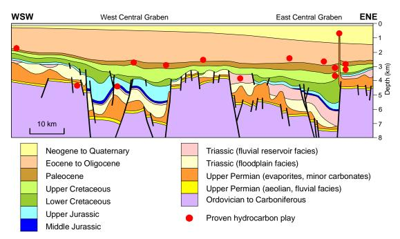
Fig. 10 Schematic section illustrating principal under-explored plays in the Central North Sea. See Fig. 4 for locations
