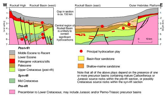
Fig. 24 Schematic play diagram for the Rockall Basin. See Fig. 21 for location
