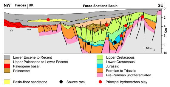
Fig. 22 Schematic play diagram for the Faroe-Shetland Basin. See Fig. 4 and 21 for location
