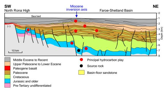
Fig. 23 Schematic play diagram for the south-western part of the Faroe-Shetland Basin. See Figure 21 for location
