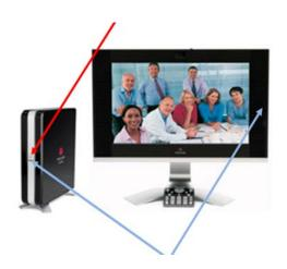
2. Press the POWER button on the side of the monitor.
