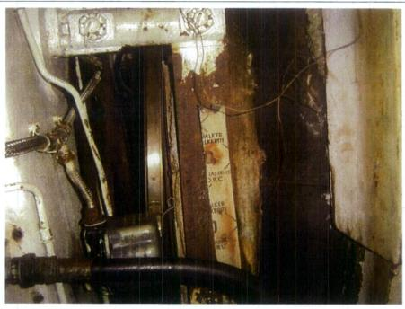
Material Comments: Asbestos containing gasket exposed to side of 1 No. engine. Suspect same gasket material is concealed within both engines
