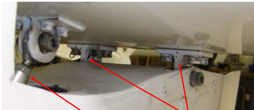
Pitch Control Input Rod Tailplane attachment lugs
