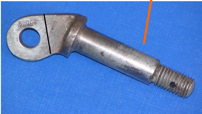
Tiger Moth Main Undercarriage drag strut showing location of failed pin and approximate line of fracture.
