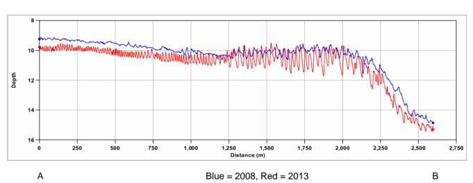
Note: the 2008 surface has been created from 10 metre density shoal biased points. The 2013 surface is a 1 metre resolution CUBE surface, with better definition of small scale features.
