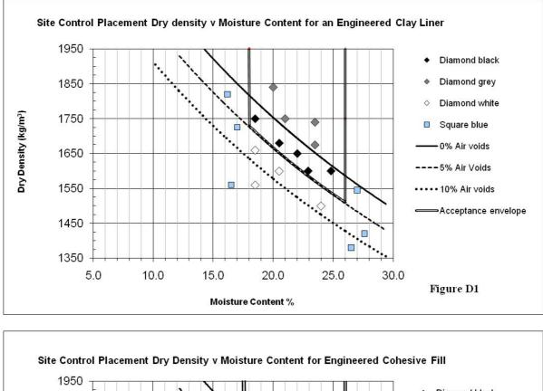
This requires that shear strength (and possibly settlement)/moisture content and density relationships are adequately defined during the source evaluation/soil characterisation phase ie before site works commence in a timely manner.
