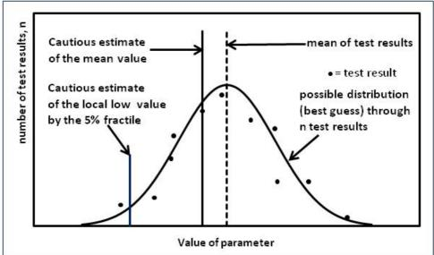
Figure B2 – Derivation of characteristic values using statistics
