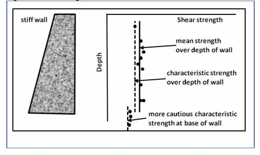
Figure B1: Retaining wall - characteristic values
