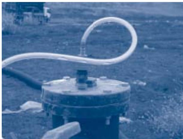
Figure 5.5 Condensate in connection tubing during sampling
