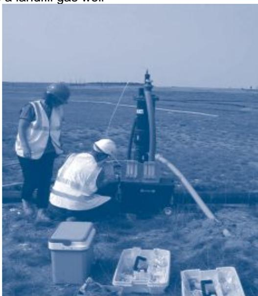
Figure 5.3 Sampling tubes and rotameter assemblies
