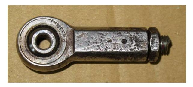
**Figure 2** G-BTAM right aileron control rod eye end with fractured threaded shank
