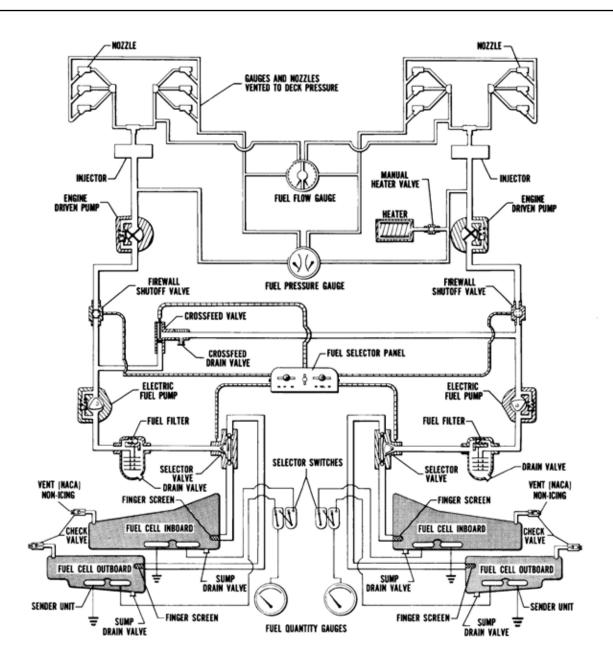
Figure 1 PA-31-310 Fuel System Schematic
