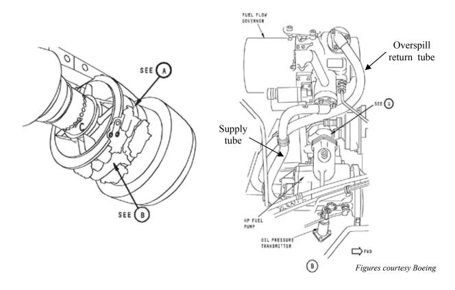
**Figure 1** Location of the HP fuel pump and FFG on the RB211-535E4 engine
