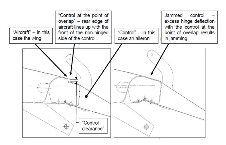
**Figure 1** Illustration of a normal and jammed control, taken from JSB 019-2
