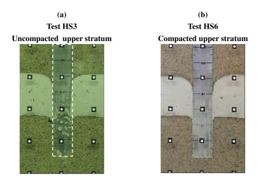
Figure 4.5. Photographs of half-section models: H-section piles
