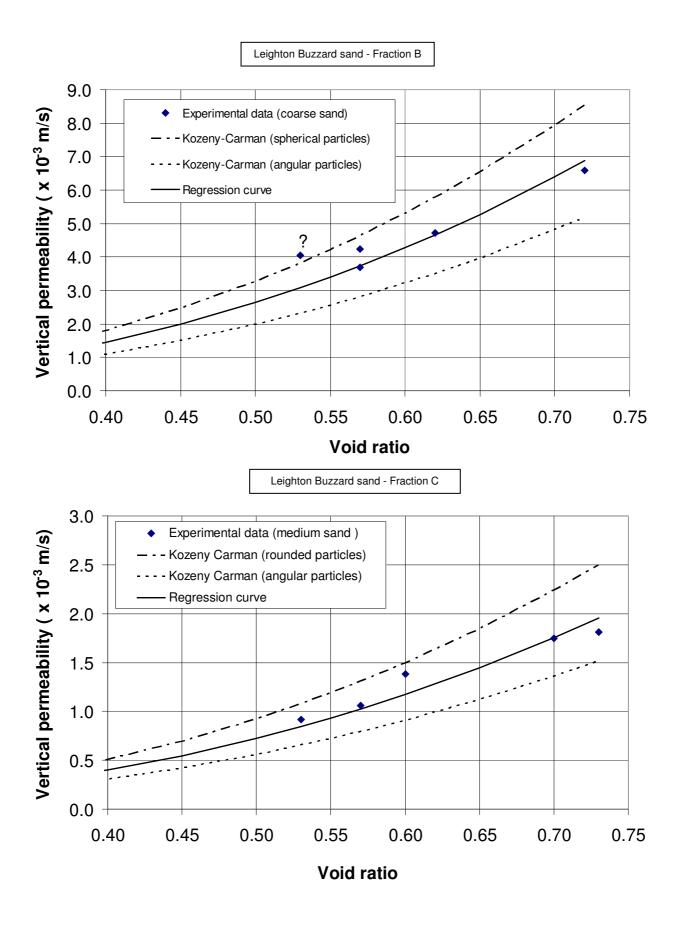
Figure 4.15. Permeability variation with void ratio for sands used in the models
