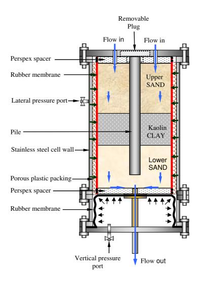
Figure 3.1. Schematic diagram of axisymmetric test configuration
