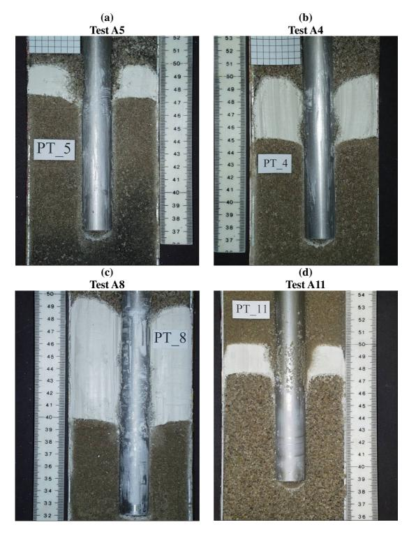
Figure 4.1. Photographs of dissected axisymmetric models: cylindrical piles
