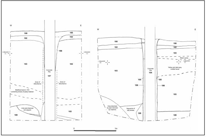
Figure 5.5. Sections showing disturbance caused by driven and pre-augered driven concrete piles at Lincoln. Numbered zones (except 104 and 107) represent various soils.
