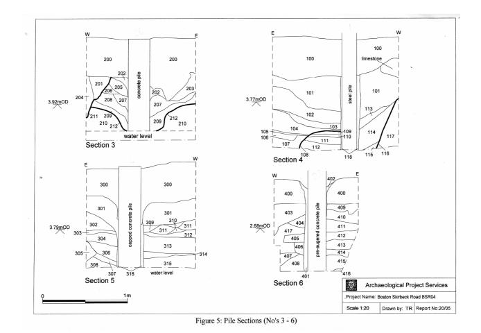
Figure 5.6. Sections showing disturbance caused by driven concrete, capped concrete and steel piles and pre-augered concrete piles at Boston (copyright Archaeological Project Services). Numbered zones represent various soils.
