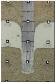
Figure 4.4. Photographs of half-section models: cylindrical piles
