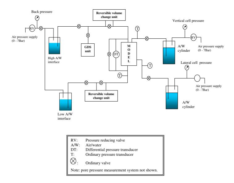
Figure 3.4. Hydraulic circuits for permeability testing
