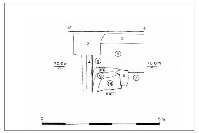
Figure 5.1. Section showing disturbance due to a pile at Barclaycard Marefair Northampton (reproduced by permission of the Historical Environment Team, copyright Nothamptonshire County Council). Zone 2 represents the pile cap, zone 4 represents the pile and the remaining zones represent various soils.
