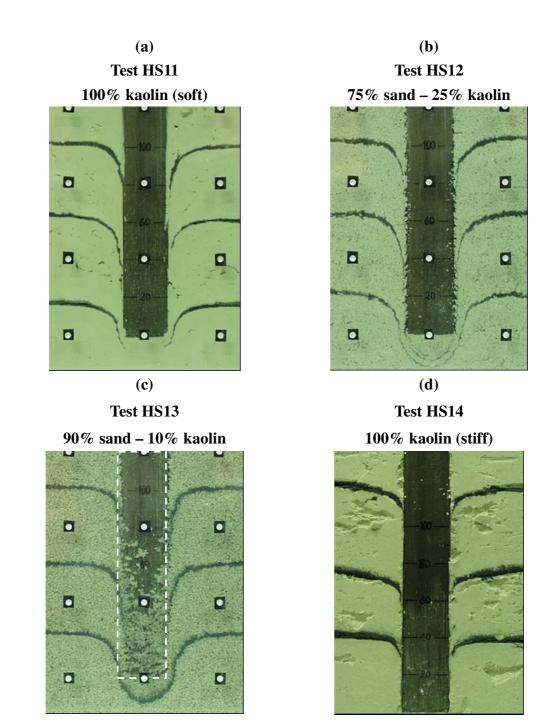
Figure 4.8. Photographs of half-section models: square piles in homogeneous soil
