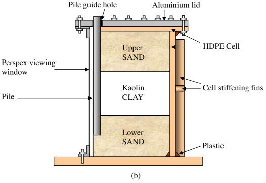
Figure 3.5. Schematic diagrams of half-section test configuration: (a) plan and (b) section
