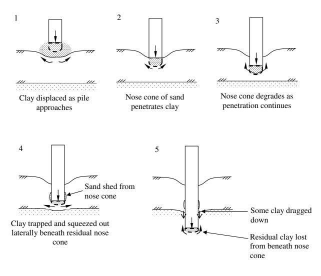
Figure 4.12. Schematic diagram of penetration stages in layered soil
