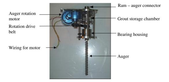
Figure 3.3. Model CFA piling equipment
