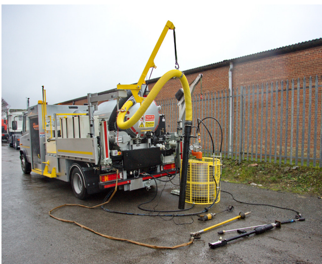
Figure 1 - Specialist equipment for core and vac operations
