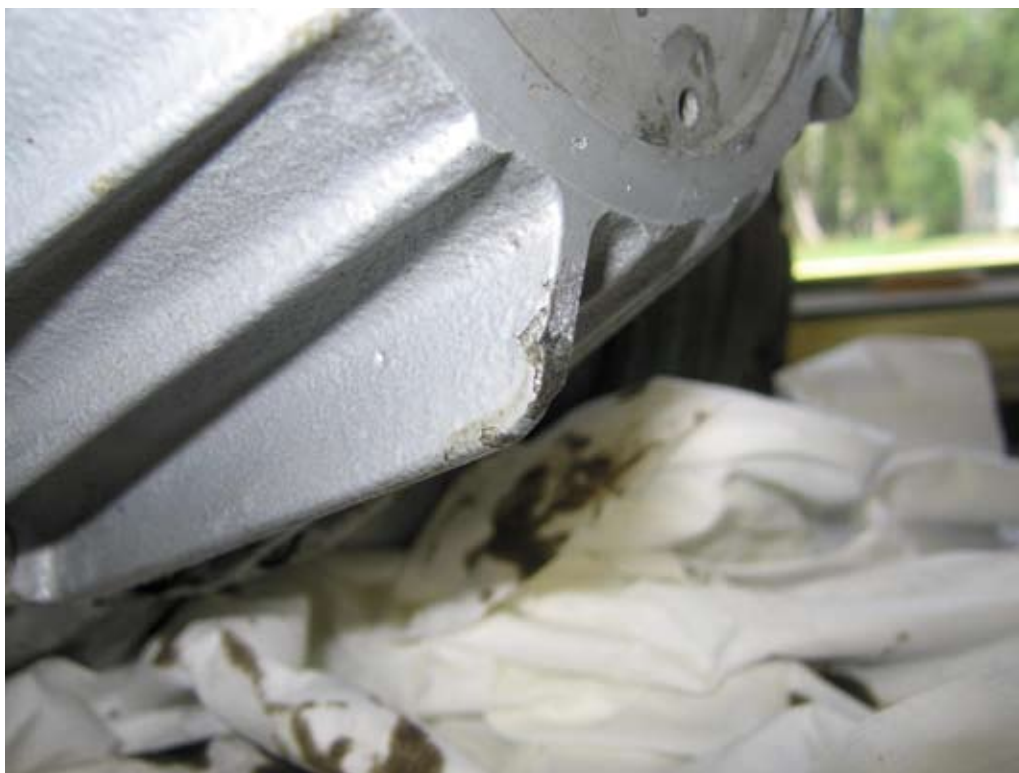
Figure 4 (right) Damaged stiffening rib
