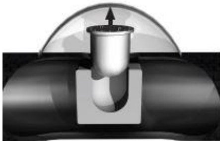
RPV is lifted out of Submarine
