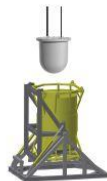
The Container lid is removed and RPV is loaded into container
