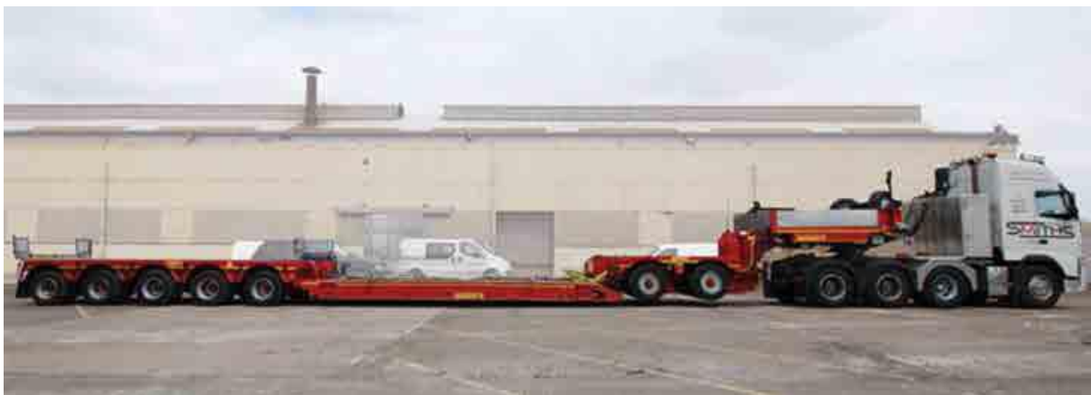
Example of type of lorry suitable for RPV transport
