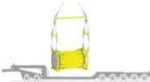
The Container is lifted onto transport trailer
